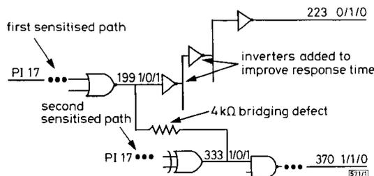
Fig. 1 Portion of the ISCAS85 c432 benchmark schematic diagram II showing a bridging defect
