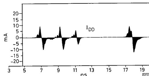
Fig. 3 Current SW of supply rail of c432 in presence of bridging defect
