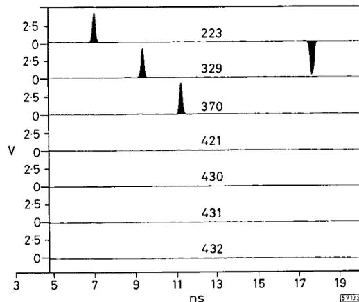
Fig. 2 Voltage SWs of seven POs of c432 in presence of bridging defect
