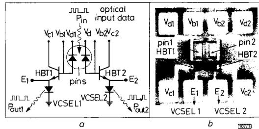
Fig. 1 Circuit design and device layout of a reconfigurable binary switching node, consisting of two individually addressable pin/HBT/VCSEL switches
