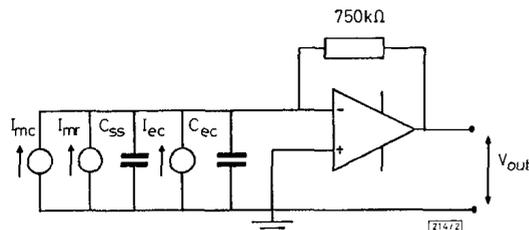
Fig. 2 Secondary sense equivalent circuit
