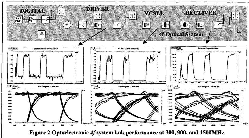
Figure 2 Optoelectronic 4f system link performance at 300, 900, and 1500MHz
