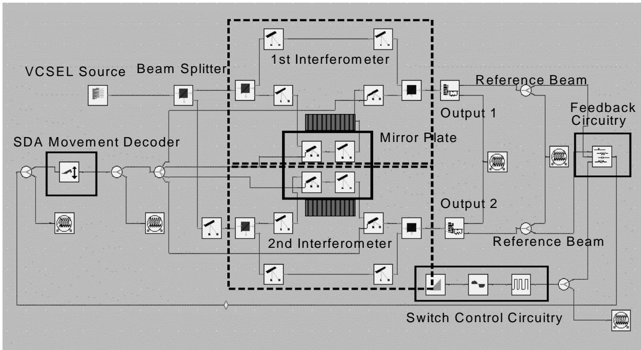
**Figure 9 1x2 Interferometer switch**
