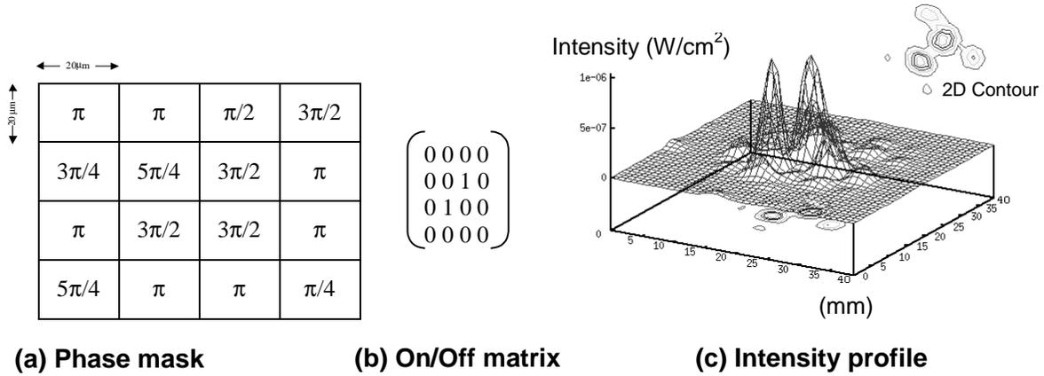
Figure 4 Plane wave propagation through a phase mask
