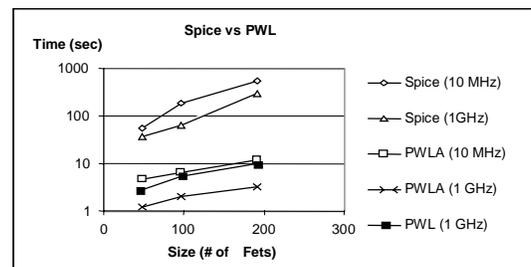
Figure 6 Spice vs. PWL and PWLA models in a system of multiple FETs (f=100/500/1000 MHz).
