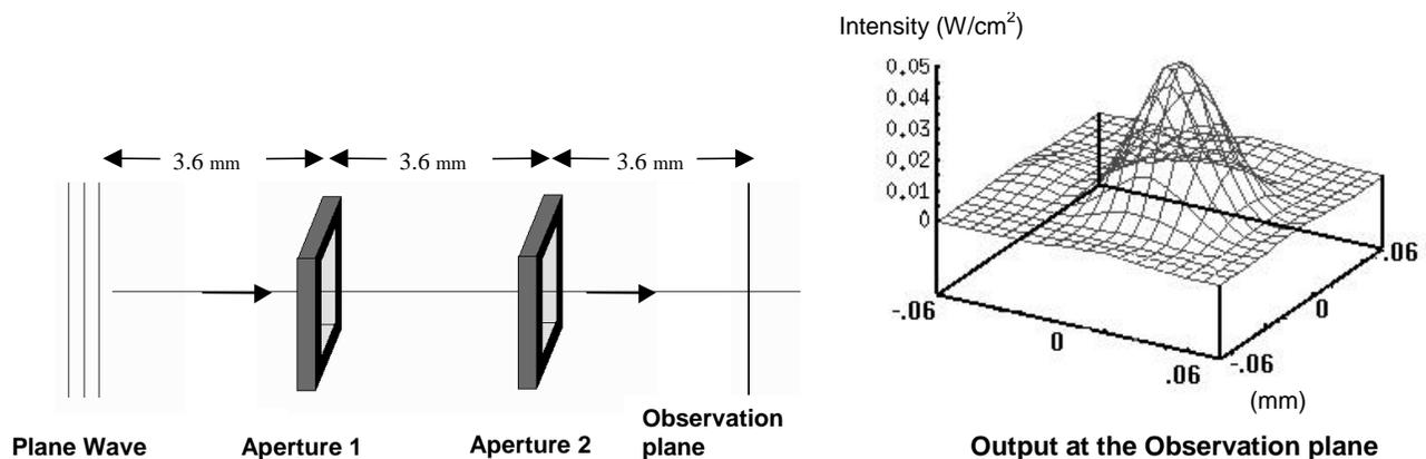
Figure 3 Plane wave propagation through cascaded apertures
