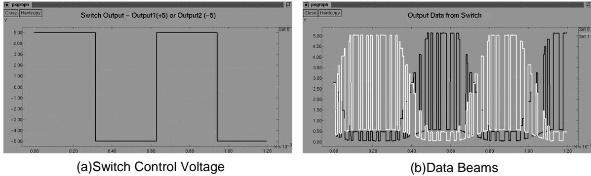
**Figure 10 Dynamic simulations of 1x2 interferometer switch**
