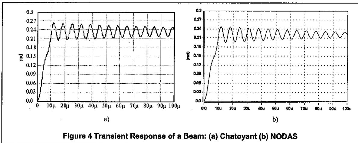
Figure 4 Transient Response of a Beam: (a) Chatoyant (b) NODAS
