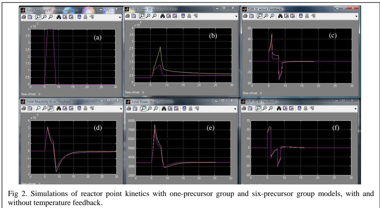
Fig 2. Simulations of reactor point kinetics with one-precursor group and six-precursor group models, with and without temperature feedback.
