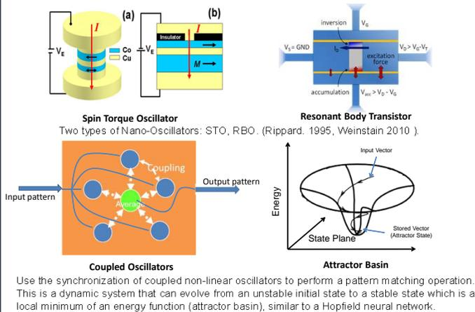
Model the coupled oscillator cluster using the Belousov-Zhabotinsky reaction model (Asai et al. 2004 ). This non-linear oscillator model can be implemented in hardware with two op-amps in a feedback loop. Simulate a cluster of coupled oscillators using these equations in Matlab and observe the synchronization.
