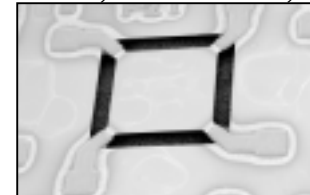
Thick-Film PZT Sensing Element University of Southampton Institute of Transducer Technology - http://www.usitt.ecs.soton.ac.uk/
