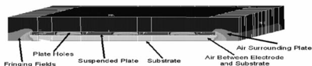
Figure 8: ANSYS Capacitance Extraction
