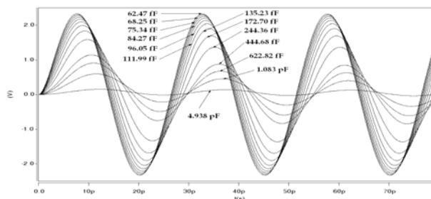
Figure 12: Switch Analysis with Variable Capacitance
