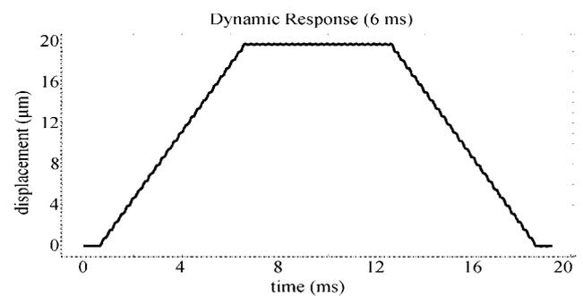
**Figure 5: Switch Response - 6ms Rise Time**
