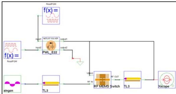
**Figure 13: Chatoyant Schematic of Full System**
