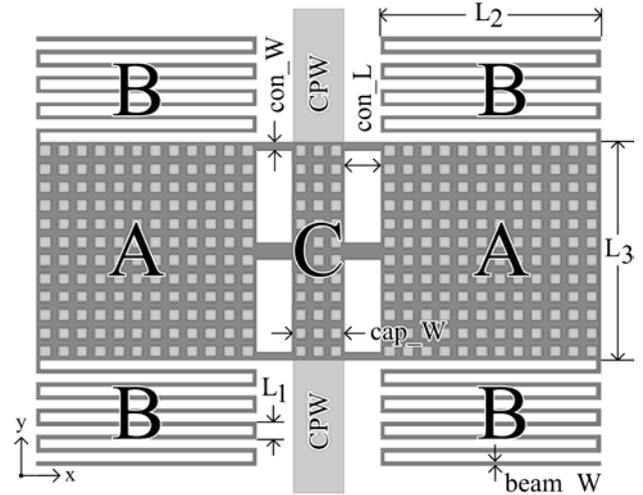
Figure 3: Schematic of RF Shunt Switch
