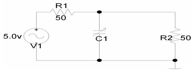
Figure 11: Circuit Schematic of RF MEMS System
