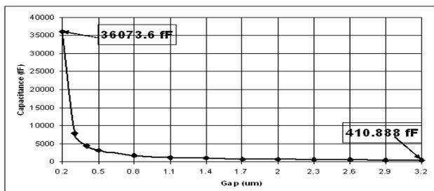
Figure 9: ANSYS Capacitance vs Stroke
