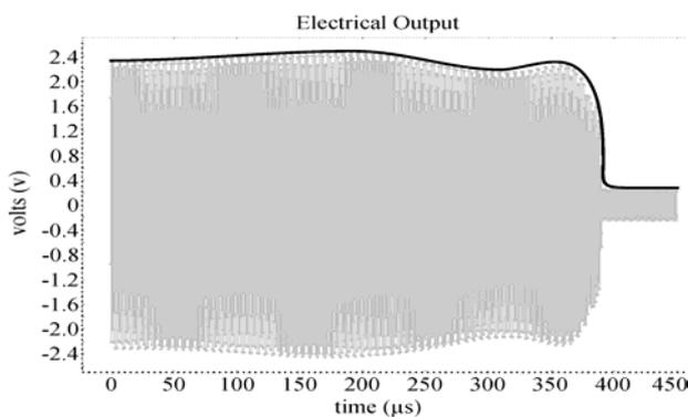
**Figure 14: Transient Response of RF MEMS Switch**
