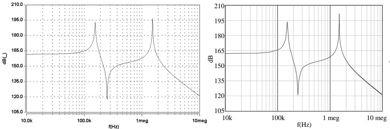
Figure 6: Frequency Response of a Beam: (a) NODAS (b) Chatoyant
