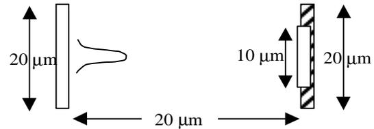
Figure 2: Gaussian Propagation Example System
