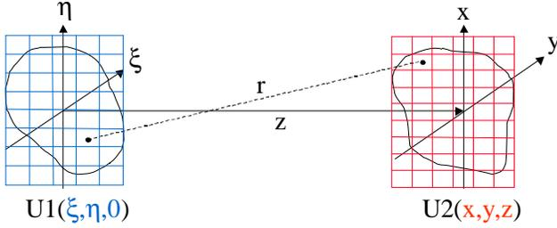
Figure 1: Aperture and Observation Coordinate System
