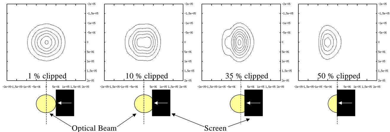
Figure 4: Intensity Contours of Clipped Gaussian Beam
