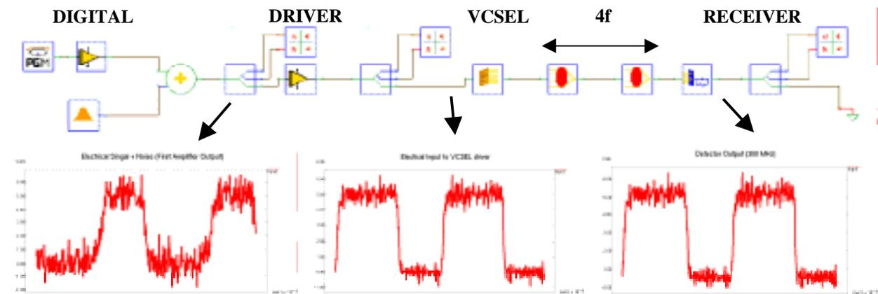
Fig. 5, Chatoyant's screen shot showing a 4f OE link system including PWL drivers and detector.
