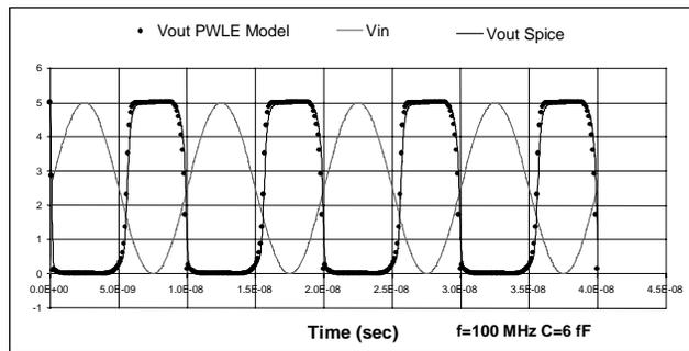
Fig. 2. PWLE and Spice output graphics under capacitive load and frequency of 100 MHz
