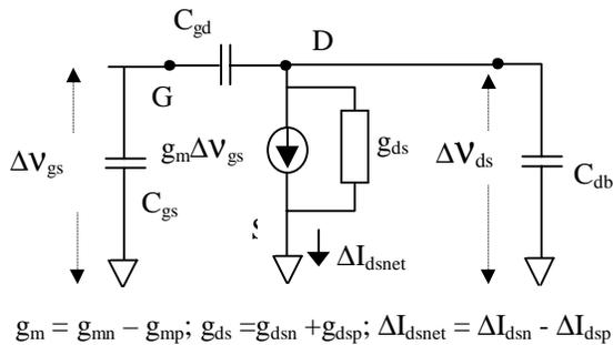
Figure 1, piecewise lineal model for the CMOS Inverter
