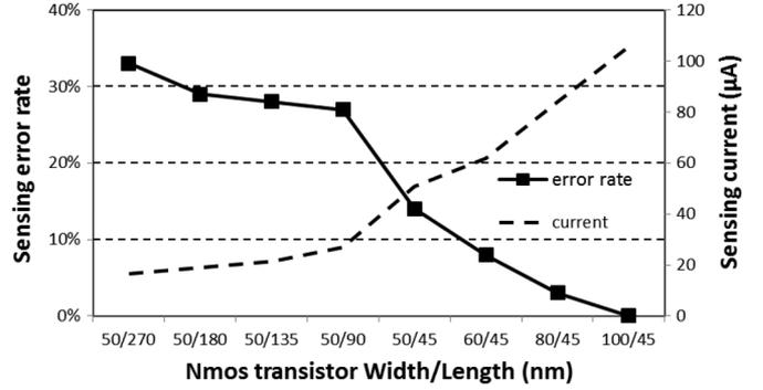
Fig. 10. Tradeoff between read disturbance probability and sensing errors of nonvolatile flip-flop when the transistor size varies.
