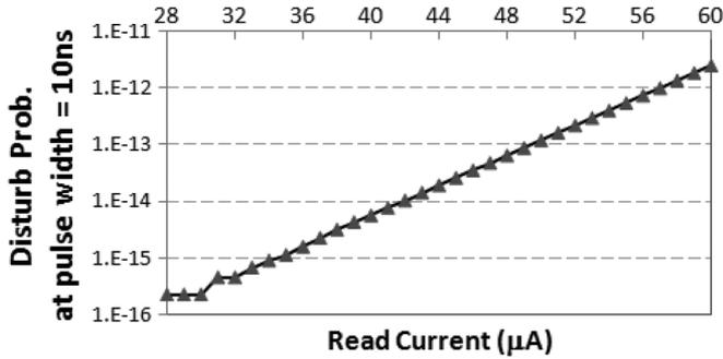
Fig. 5. The variations of MTJ read disturbance probability when read current amplitude changes.
