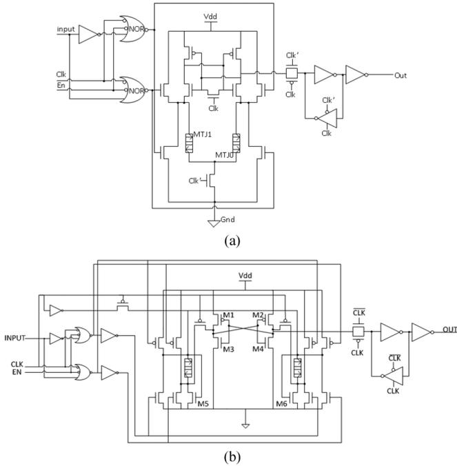
Fig. 8. Nonvolatile flip-flop designs. (a) Original design in [1]. (b) Our modified design.
