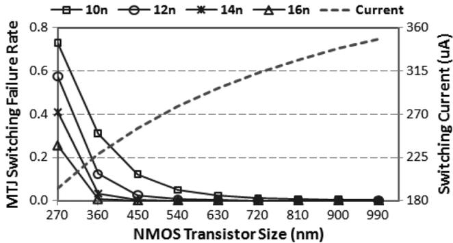
Fig. 6. The nonpersistent failure rate of MTJ as the transistor size varies.
