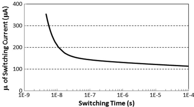
Fig. 2. Relationship between MTJ switching time and switching current.
