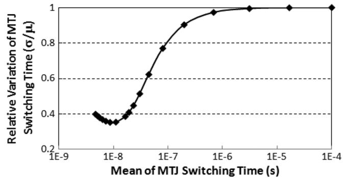
Fig. 4. Variations of MTJ switching time due to thermal fluctuations.
