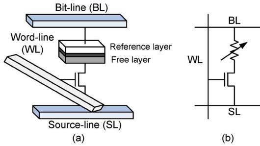
Fig. 1. 1T1J STT-RAM cell. (a) Cell view. (b) Equivalent schematic.
