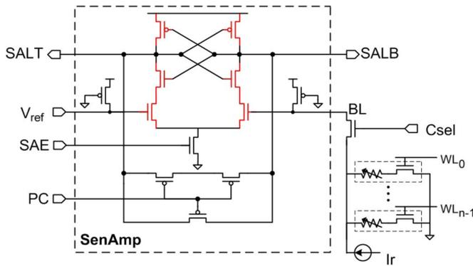
Fig. 3. Conceptual sense amplifier design.
