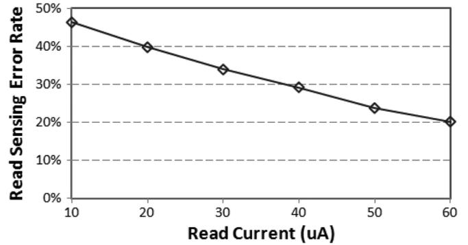
Fig. 7. Tradeoff between read disturbance probability and sensing errors.
