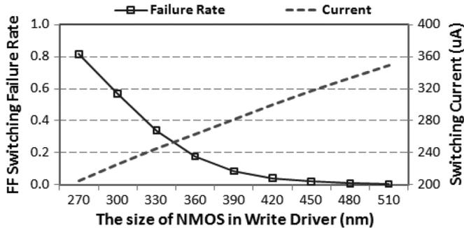
Fig. 9. The nonpersistent write failure rate of nonvolatile flip-flop when the transistor size varies.
