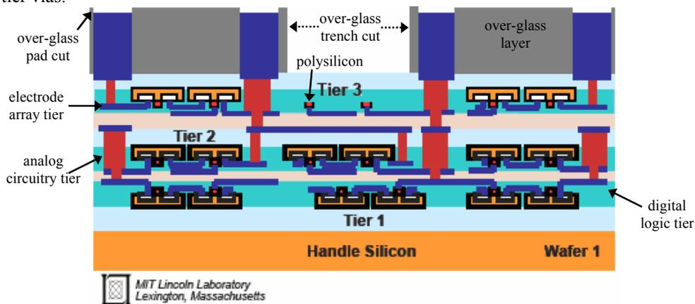
Fig. 1. Cross section of 3D chip stack (Courtesy of MIT Lincoln Laboratory, used with permission). Displayed on each chip tier are the active silicon and interconnect layers. The center over-glass cut is an example of how the over-glass layer can be used to form fluidic trenches. Figure not drawn to scale.
