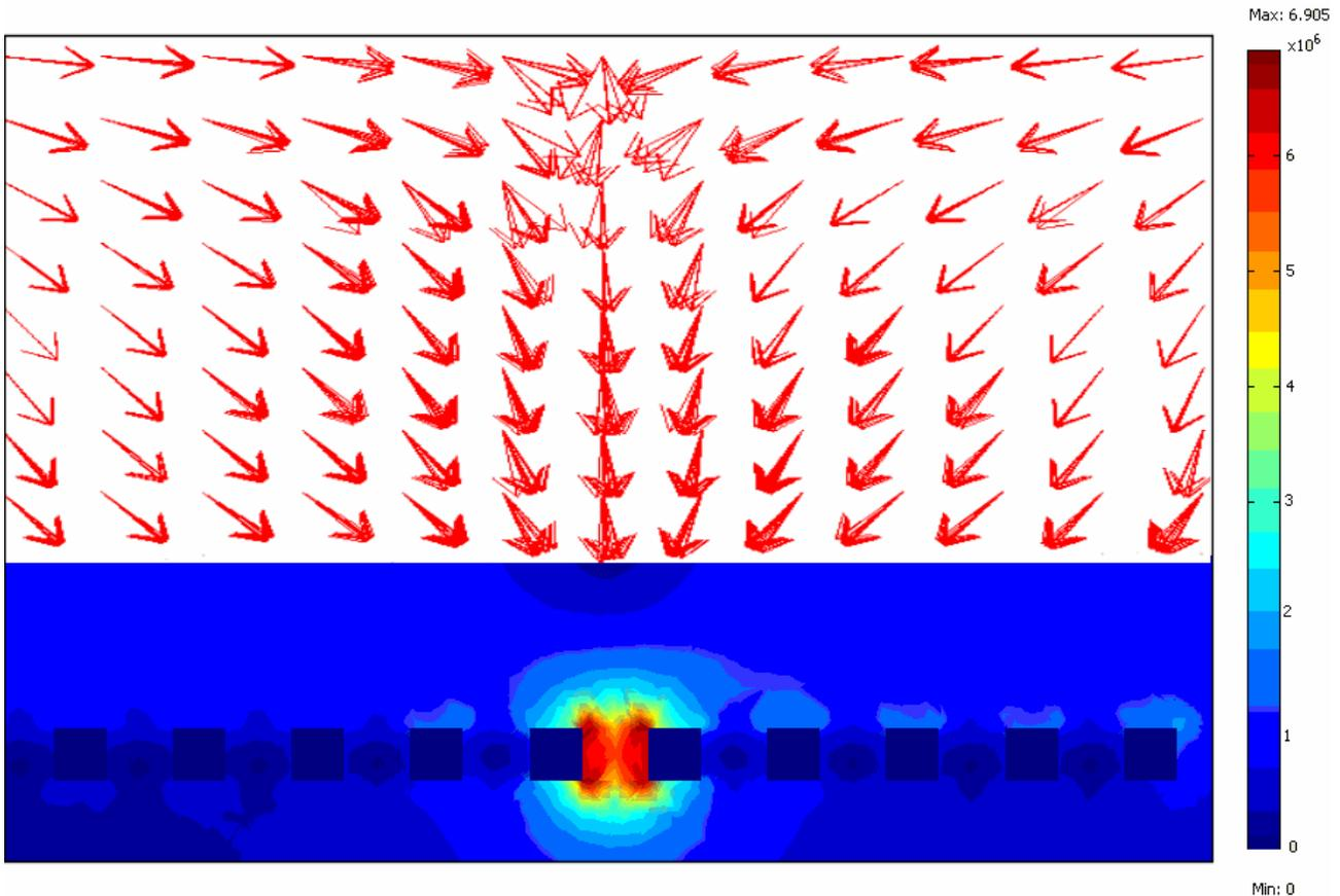
Fig. 6. Finite element analysis of electric field and resulting dielectrophoresis force vectors due the voltage on the center two electrodes being out of phase with each other.
