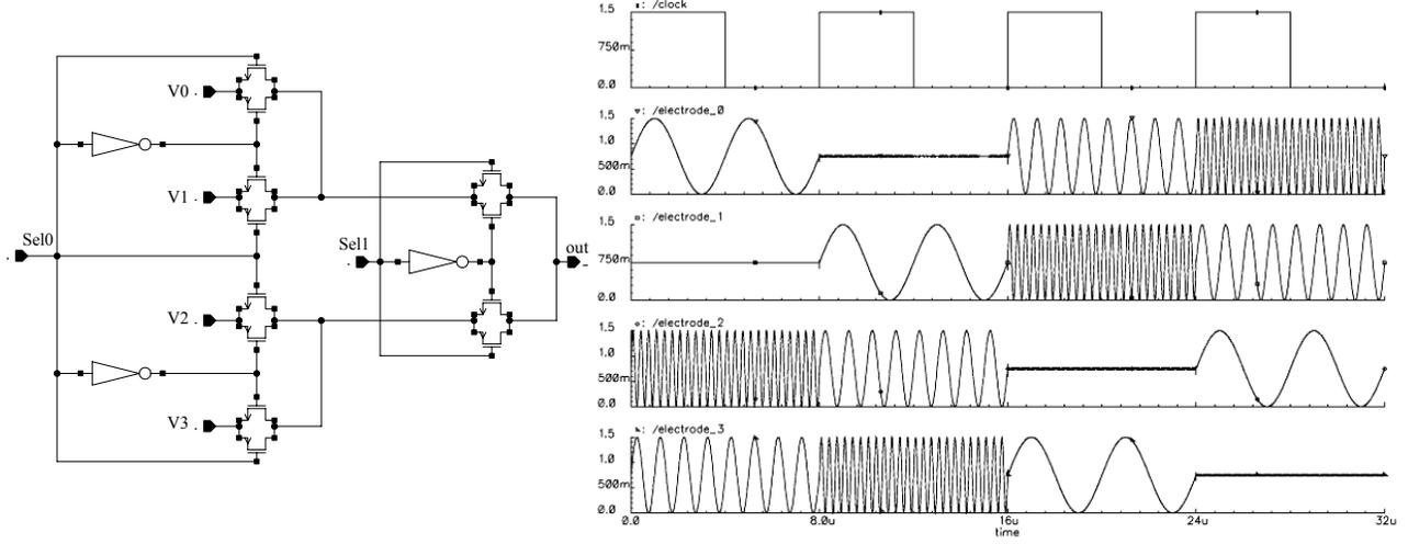
Fig. 4. The left shows one of the 4:1 analog multiplexers, on the right are simulation results of four such muxes switching the waveform on four separate electrodes on the rising edge of every clock cycle.
