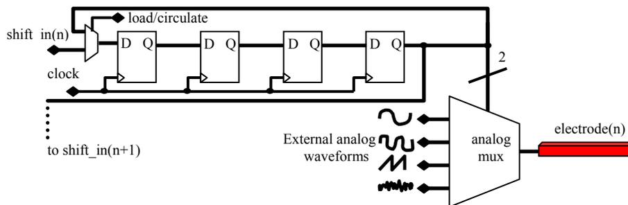
Fig. 3. Block diagram of circuitry used to control each electrode. The circular shift register selects which of the four external waveforms will appear on the electrode. The output of the shift register is also used as the input to the shift register on the successive row when initializing the selection pattern.
