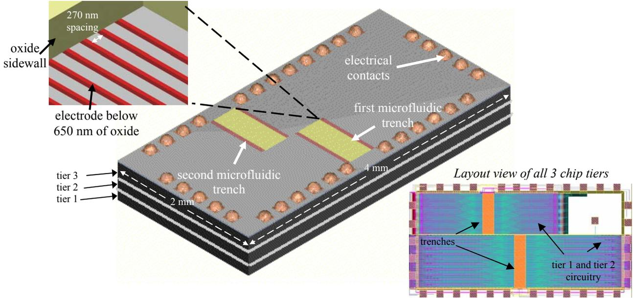
Fig. 2. Physical layout of 3D lab-on-chip. The top tier is used for fluid trenches and polysilicon electrodes. Analog and digital circuitry is located on the middle and bottom chip tiers. Inset at top shows a close-up of the polysilicon electrodes. The bottom inset shows a superposition of the VLSI layout of all three chip tiers.
