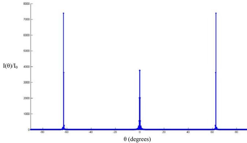
Fig. 9. Distribution of light intensity diffracted by grating formed of particles trapped by dielectrophoresis with  $d=250$  nm,  $a = 450$  nm,  $N = 2,048$  and  $\lambda=400$  nm
