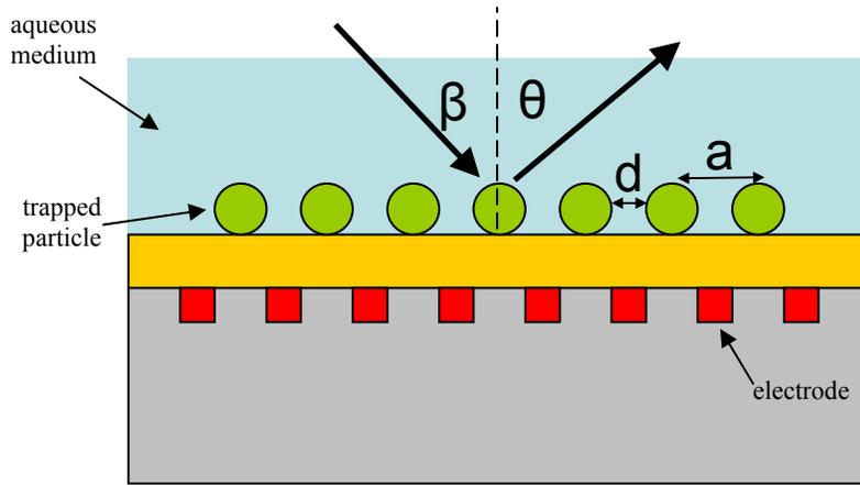
Fig. 8. 2D cross section of dielectrophoretically trapped particles arranged to form a diffraction grating
