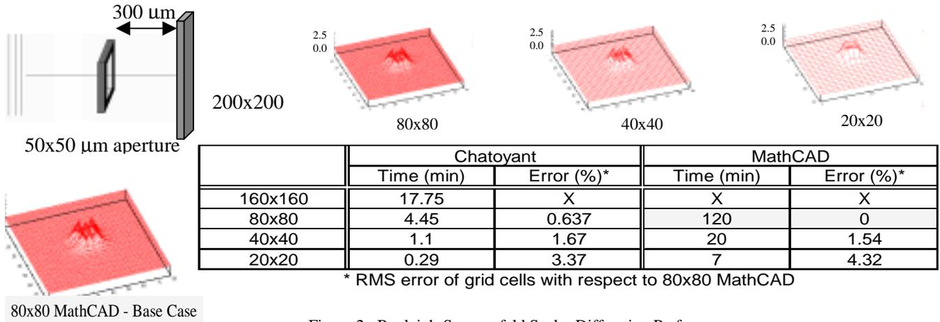
Figure 2: Rayleigh-Sommerfeld Scalar Diffraction Performance
