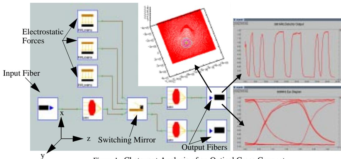
Figure 1: Chatoyant Analysis of an Optical Cross Connect
