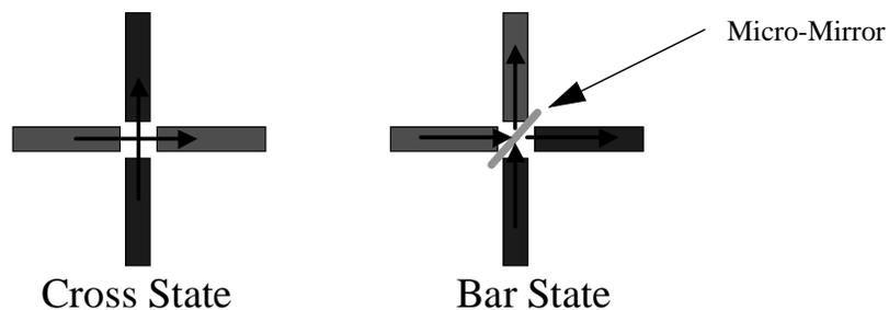
Figure 5: 2x2 Switch: Cross and Bar State
