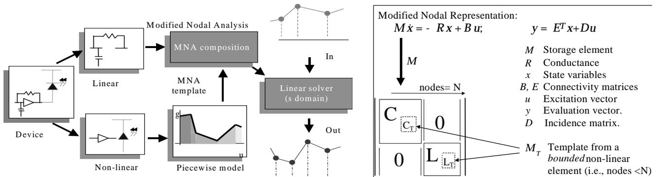
Figure 3: (a) Piecewise Modeling Technique (b) MNA Representation and Template Integration
