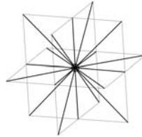
**Figure 2.** Single node from a three-dimensional LSM system; six orthogonal and twelve diagonal bonds can be seen
