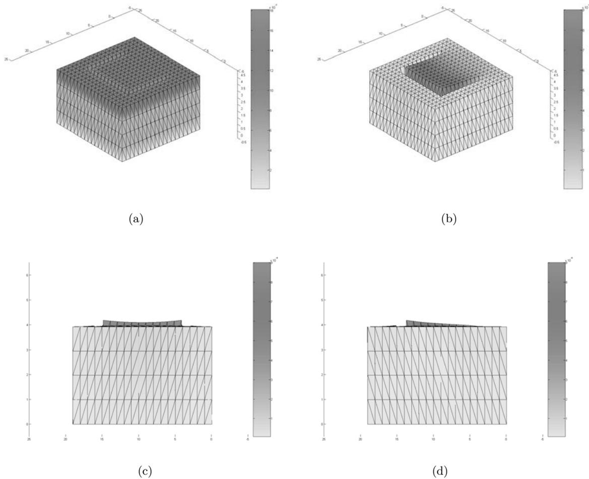
**Figure 5.** Forced cut, ‘Tongue’ configuration – (a) Surface prior to simulation; (b) Surface after simulation; (c) Surface after simulation as viewed from front; (d) Surface after simulation as viewed from near side
