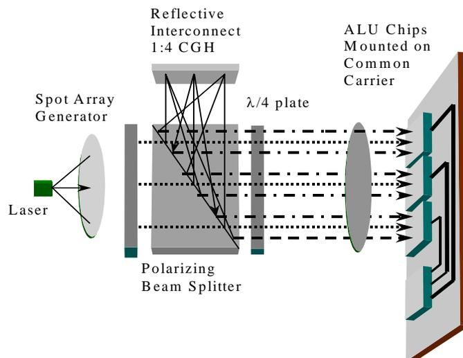
**Figure 3: Optical Setup**
