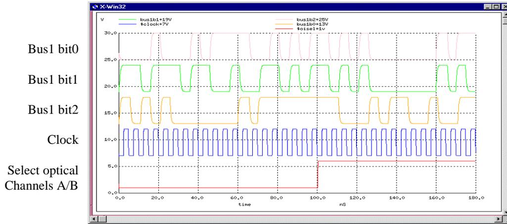
Figure 4: Electrical Simulation, optics in to optics out at 200Mhz
