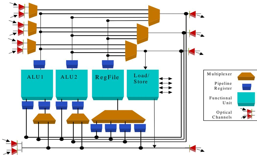
**Figure 2: Single Chip Architecture**
