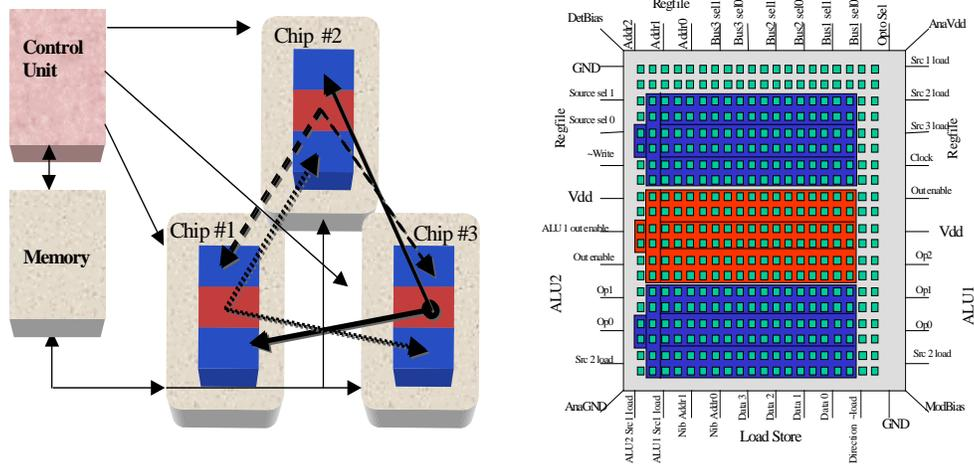
Figure 1: Optical Bus Layout and Optoelectronic Interface
